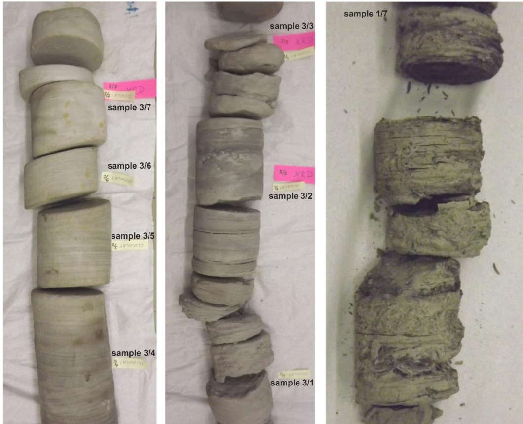
Figure S2: Typical lithologic characters of the analyzed core sections (core diameter: 76 mm). (a) Alternating fine-grained sandstones and siltstones with disseminated pyrite (brown spots), core #3. (b) Alternating very fine-grained sandstones and mudrocks, core #3. (c) Coal-bearing claystones, core #1.
