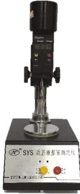
(a) Liquid-plastic limit tester
