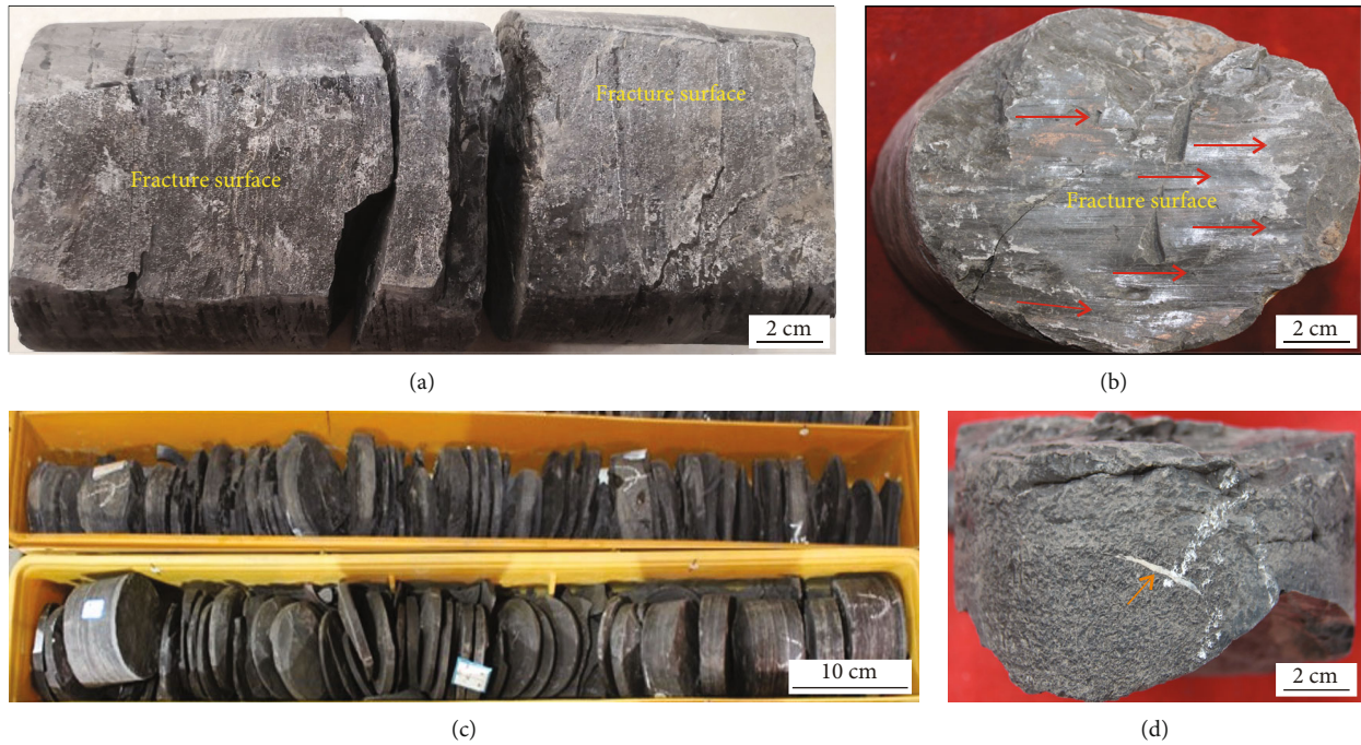
FIGURE 3: Fracture types and characteristics in shale oil reservoirs of Qing-1 Member. (a) Extension fracture with high dip angle, and partially filled with calcite. Well G53, 1945.62 m. (b) Shear fracture with moderate dip angle, red arrows indicate striations and sliding directions. Well G47, 1986.27 m. (c) Closely spaced bedding-parallel fractures. WG81, 1845.10-1847.00 m. (d) Overpressure fracture (where the orange arrow indicates). Well G13, 1994.56 m.
