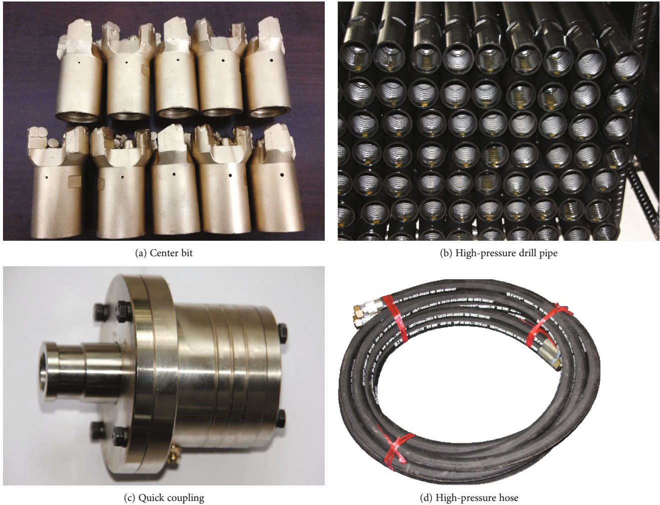
FIGURE 6: Main components and physical drawing.
