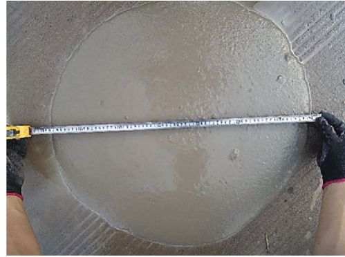
FIGURE 1: Test of slump flow.
