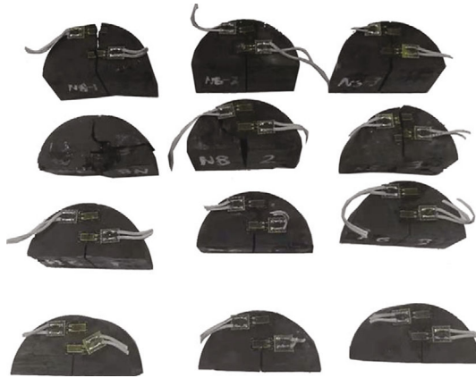
FIGURE 10: Failure mode of samples in the NSCB test.
