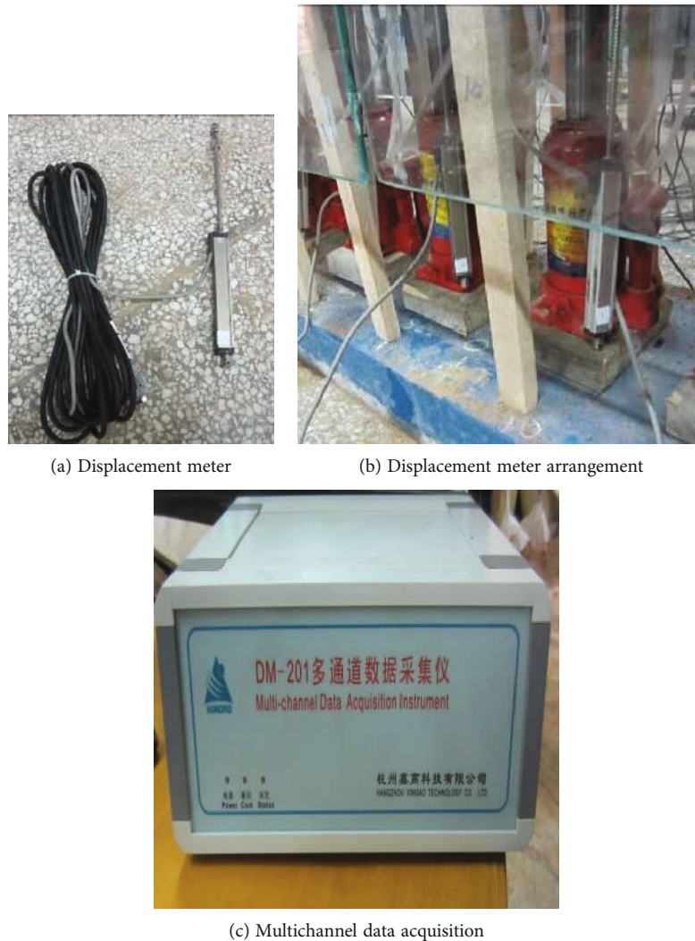
FIGURE 2: Monitoring instruments and its arrangement for soil subsidence.
