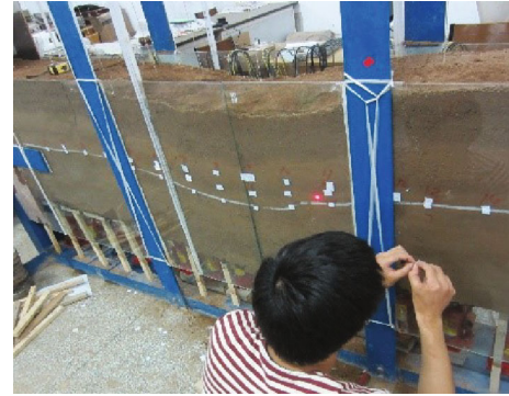
FIGURE 4: Observation of settlement of soil in pipeline layer.
