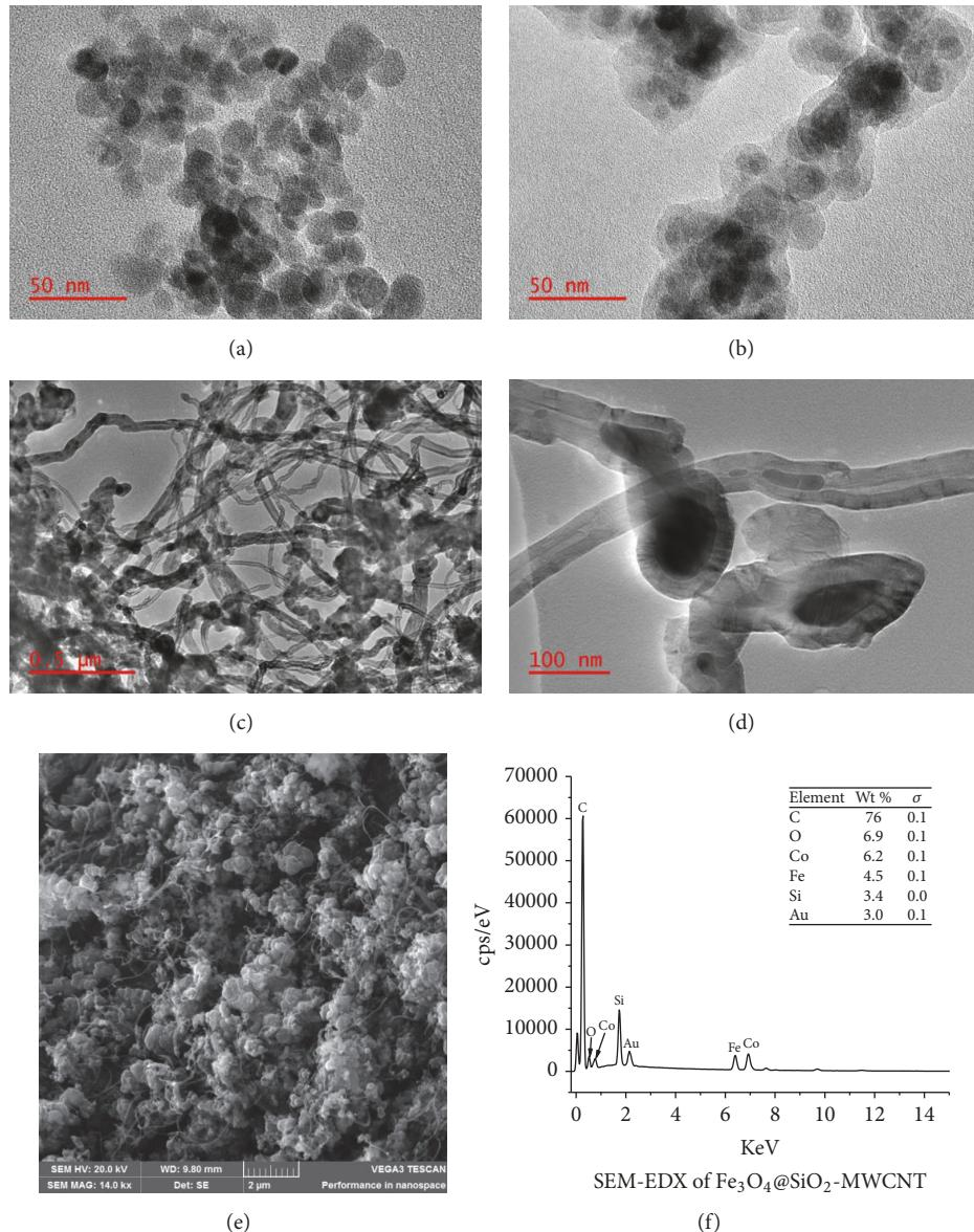
FIGURE 1: TEM image of  $\text{Fe}_3\text{O}_4$  (a),  $\text{Fe}_3\text{O}_4@\text{SiO}_2$  (b),  $\text{Fe}_3\text{O}_4@\text{SiO}_2\text{-MWCNT}$  (c-d), SEM image of  $\text{Fe}_3\text{O}_4@\text{SiO}_2\text{-MWCNT}$  (e), and SEM-EDX of  $\text{Fe}_3\text{O}_4@\text{SiO}_2\text{-MWCNT}$  (f).
