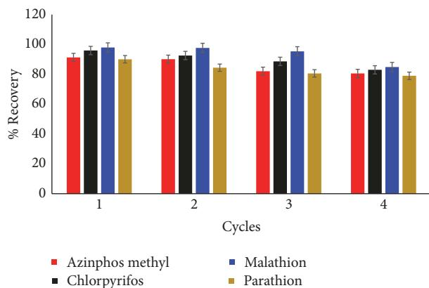
FIGURE 8: Recycling and reuse of the  $\text{Fe}_3\text{O}_4@\text{SiO}_2$ -MWCNT adsorbent in the removal of azinphos methyl, chlorpyrifos, malathion, and parathion mix from aqueous solution.
