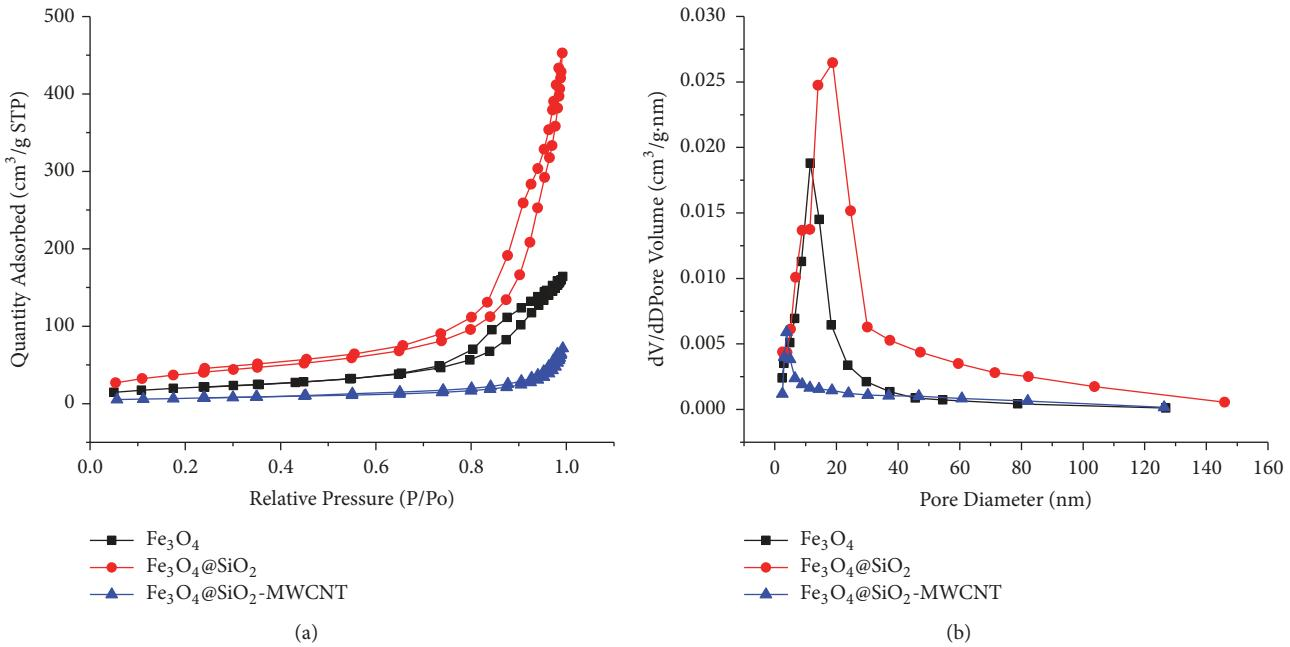
FIGURE 3: Panel (a) is the nitrogen adsorption-desorption isotherm for  $\text{Fe}_3\text{O}_4@\text{SiO}_2$ -MWCNT, and panel (b) is the corresponding PSD.
