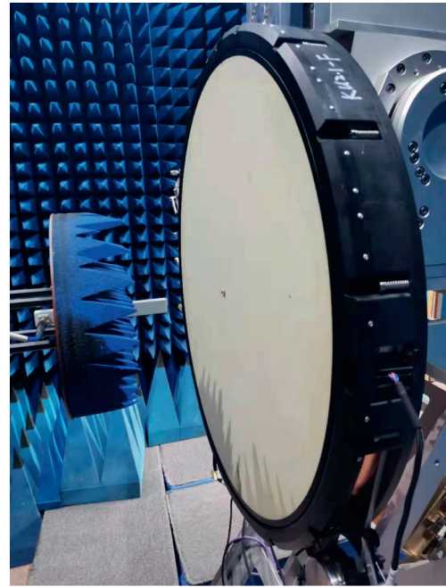
FIGURE 7: Antenna prototype and measurement system.
