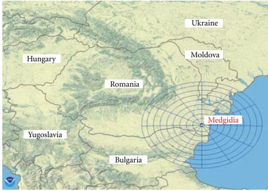
FIGURE 1: The spatial domain of radar analysis (geographic projection). The radar range is 230 km, the spatial resolution is 1 km, and the temporal resolution is 6 minutes, between two scans. NOAA Weather and Climate Toolkit (<http://www.ncdc.noaa.gov/oa/wct/>).
