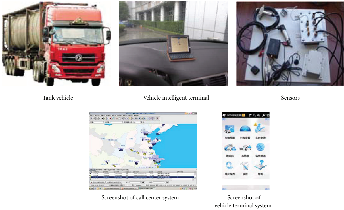
FIGURE 4: Real pictures of Electronic Fence in hazardous chemicals transport CPS.
