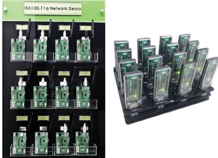
FIGURE 6: (a) Experimental network with eight ISA100.11a sensor nodes (b) Freescale MC1322X USB dongle hub.
