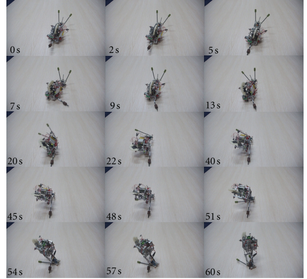
FIGURE 12: The automatic self-righting sequences of the jumping robot from front side.
