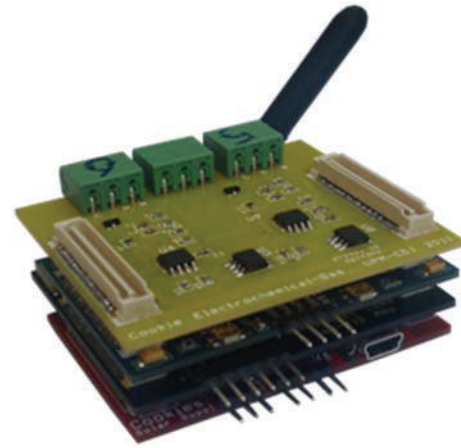
FIGURE 6: Cookie node with the electrochemical sensor board.
