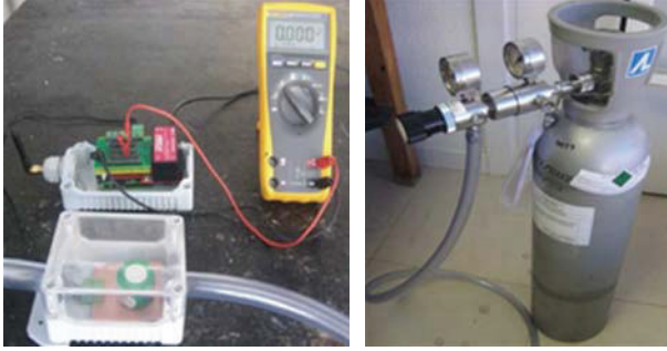
FIGURE 7: Gas calibration test conditions. Target gas: carbon monoxide. Sensor: CO-BF (Alphasense). Concentration: 300 ppm. Volume: 5 mL/min. Temperature: 25°C.
