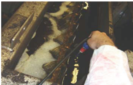
FIGURE 19: Sewage plant. pH sensor.
