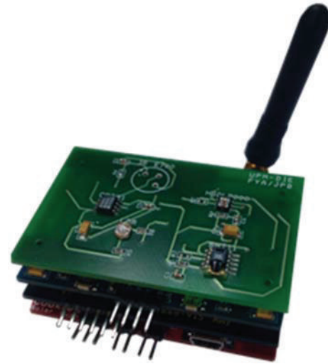
FIGURE 9: Sensor node. SHT11 based.
