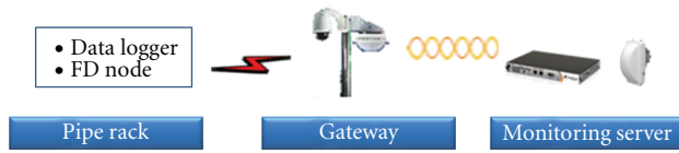
FIGURE 5: Configuration of the WSN health monitoring system for pipe racks.
