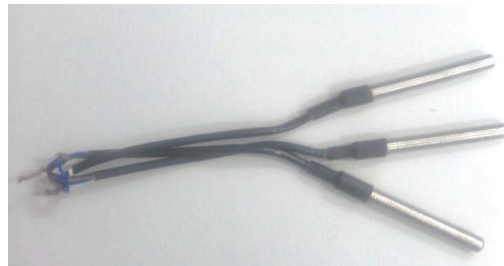
(b) Digital thermometer for internal temperature measurement of mass concrete
