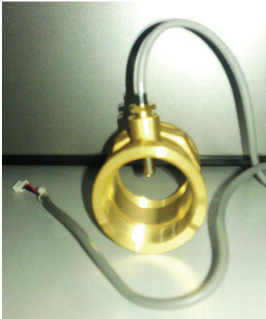
(a) Digital internal temperature measurement devices of cooling pipe
