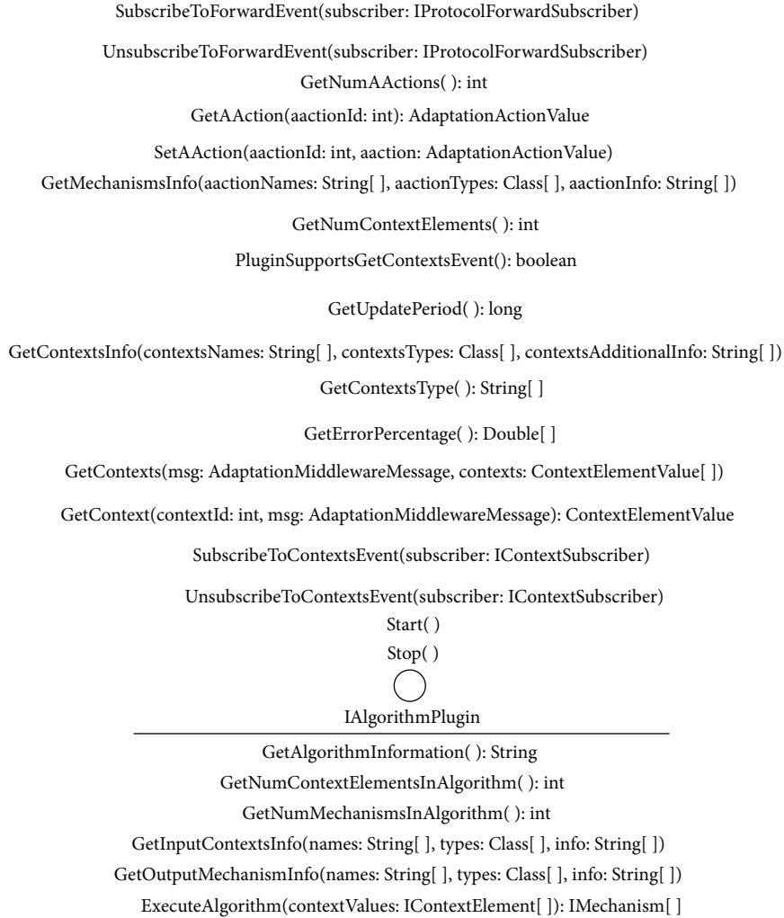
FIGURE 20: Definition of the service interfaces for all the different types of plug-ins in the PLUGAM architecture.
