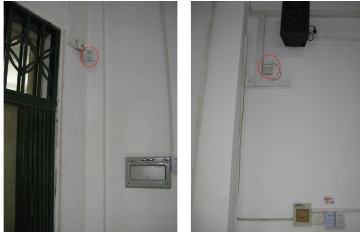
FIGURE 6: Aruba APs deployed in classrooms.
