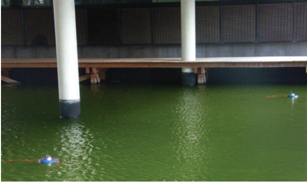
FIGURE 10: Picture of the deployment in the artificial lake at the University of Twente campus. The environment is a small lake between office buildings and consists of concrete walls and floor. The gateway node was placed near an office to allow a network connection to be made to campus network, allowing access to the testbed through internet. The nodes are kept floating with the radio antenna above the water surface, to allow a radio connection to the gateway for collecting measurement data, and are fixed with a sandbag on the floor. The acoustic transducer is deployed underwater and acoustic communication is performed through the water.
