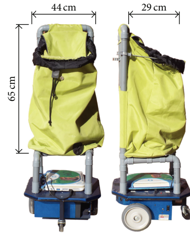
FIGURE 23: CompaRob-2 prototype: an improved version of CompaRob shopping cart based on first user usability tests and suggestions.
