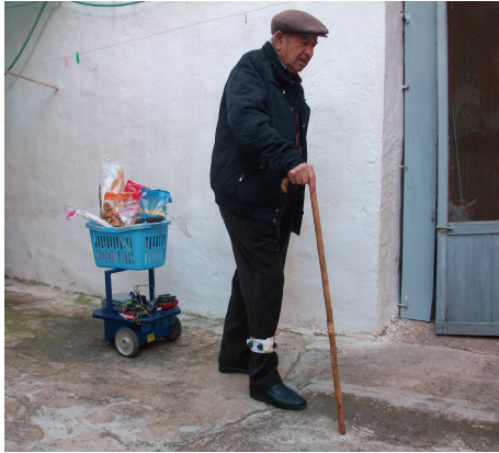
FIGURE 2: Robot following an elder person using ultrasound and radio sensors. An ultrasound ring transmitter is attached to the elder person's leg. The robot can follow the elder person using the received signals.
