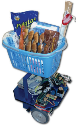
FIGURE 1: CompaRob: a person following shopping cart assistance robot based on the Erratic robotic mobile platform equipped with a shopping basket.
