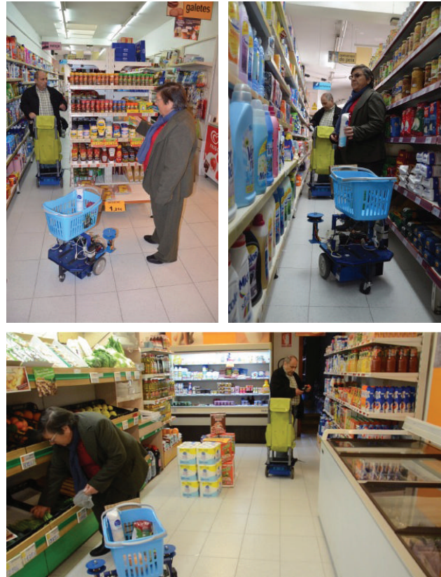
FIGURE 24: Usability tests with two robots in a larger grocery store. Both CompaRob and CompaRob-2 robots were tested with different people doing normal shopping.
