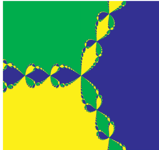
FIGURE 2: The global dynamics of F(z) = (-z^3 + 3z^2 + 1)/3z , the Newton map for f(z) = z^3 - 1 . The blue region represents A_F(1) , green represents A_F(e^{2\pi i/3}) , and yellow represents A_F(e^{-2\pi i/3}) .
