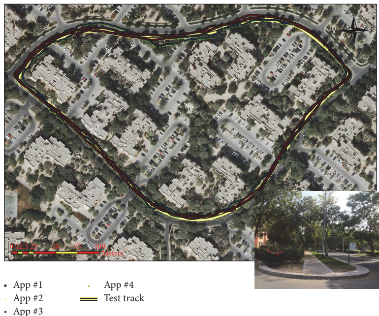
FIGURE 5: Aerial photo showing the observations that were obtained by the two devices during Test B using different smartphone applications along the same test track. It is noted that App #1 and App #2 (on iPhone) provided the same results and that App #3 and App #4 (on Samsung) provided the same results.
