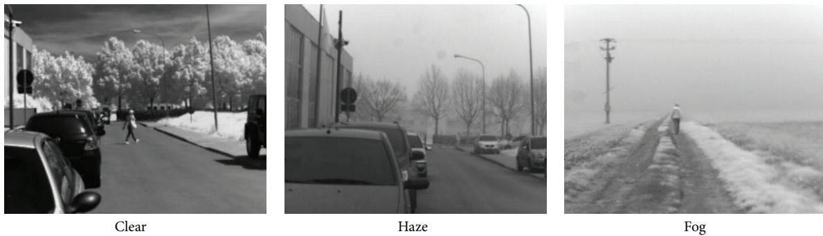
FIGURE 11: Images acquired in the SWIR spectrum (1.0 μm–1.7 μm)—filter F2—with different visibility conditions during summer, autumn, and winter, respectively.
