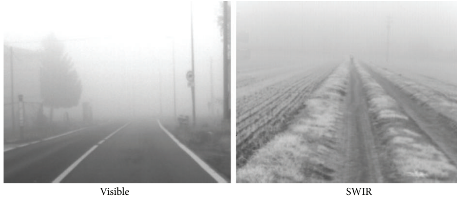
FIGURE 17: Images acquired in the visible only ( 0.4\ \mu\text{m} – 0.9\ \mu\text{m} ) and SWIR ( 1.0\ \mu\text{m} – 1.7\ \mu\text{m} ) spectrum—filter F1—respectively: with similar fog densities the scattering effect is predominant at both bandwidths so that the pedestrian walking along the country path in the SWIR image is hardly detectable.
