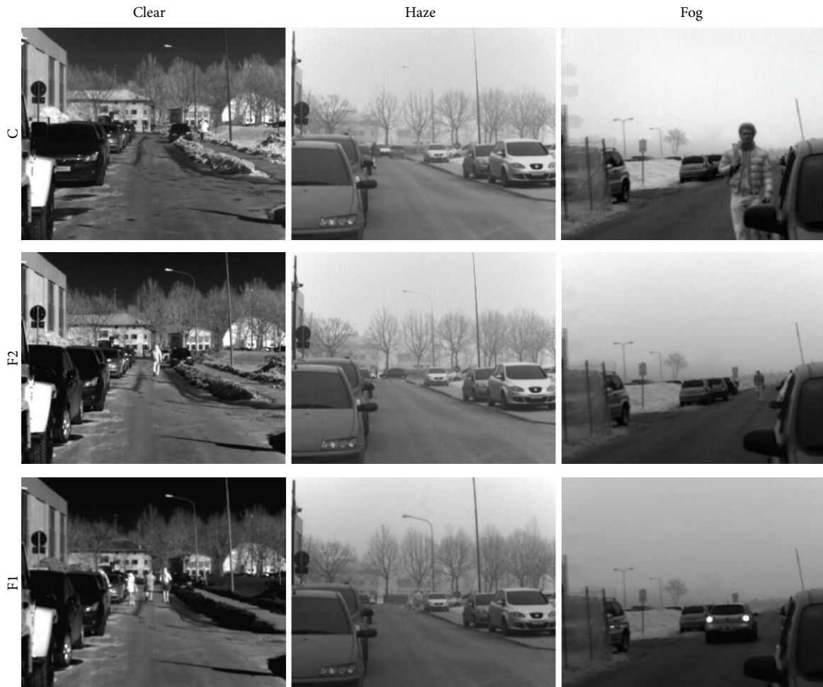
FIGURE 12: Images acquired in the whole visible to SWIR spectrum ( 0.4\ \mu\text{m} – 1.7\ \mu\text{m} )—filter C—and in the two SWIR bandwidths available on the FPA: SWIR spectrum ( 1.0\ \mu\text{m} – 1.7\ \mu\text{m} )—filter F2—and SWIR spectrum ( 1.3\ \mu\text{m} – 1.7\ \mu\text{m} )—filter F1. Acquisitions have been carried out with clear, hazy, and foggy visibility conditions, as indicated by the columns titles, and during different seasons, this having as a consequence different gain and exposure time settings to avoid image saturation. In particular, images shown in the first column appear quite dark in respect of the others as due to a very bright winter day the exposure time had been set to 1.0\ \mu\text{m} . Note that, as stated by the theory of major water absorption happening in the SWIR spectrum, in these images the snow color (low right side, adhering to the footpath curb) gets darker as the bandwidth narrows from the whole visible to SWIR spectrum to the pure SWIR ones.
