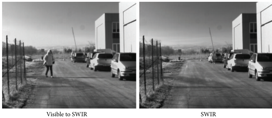
FIGURE 15: Images acquired in the whole visible to SWIR ( 0.4\ \mu\text{m} – 1.7\ \mu\text{m} ) spectrum—filter C—and in the SWIR only ( 1.3\ \mu\text{m} – 1.7\ \mu\text{m} ) spectrum—filter F1—respectively: almost invisible in the first image, the background mountains become quite clear in the second image.
