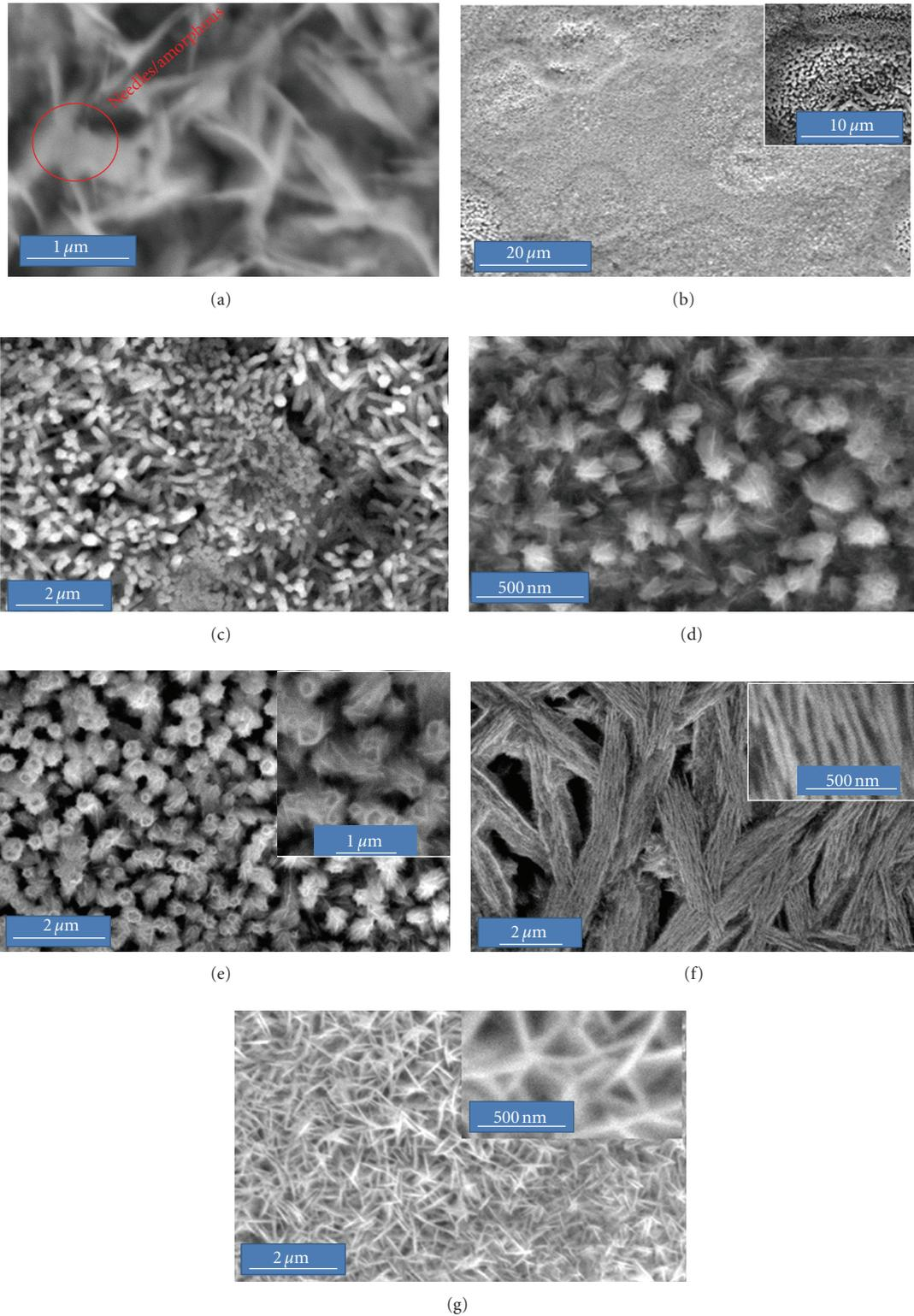
FIGURE 2: (a)  $\text{Bi}_2\text{Se}_3$  nanostructures formed at a  $T_{\text{sub}}$  of  $95^\circ\text{C}$ . (b–g): SEM images of  $\text{Bi}_2\text{Se}_3$  nanostructures synthesised at a  $T_{\text{sub}}$  of  $165^\circ\text{C}$ . Nanoparticle laden warping and cavities (b), nanorods (c), nanoflowers (d), hollow nanotubes (e), nanofibers (f), and nanoneedles (g). Insets are the close up images.
