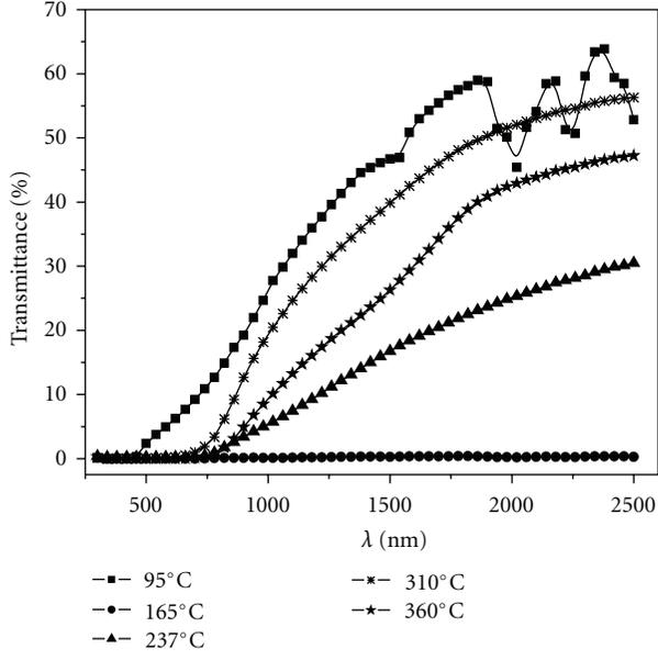
FIGURE 4: Transmittance spectra of  $\text{Bi}_2\text{Se}_3$  prepared at different  $T_{\text{sub}}$ .
