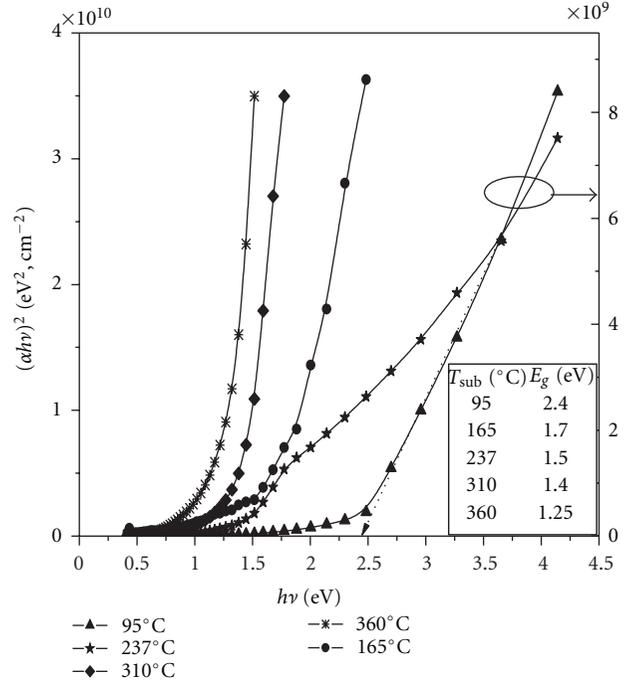
FIGURE 5: Plot of  $(\alpha h\nu)^2$  and photon energy  $h\nu$  for  $\text{Bi}_2\text{Se}_3$  prepared at different  $T_{\text{sub}}$ .
