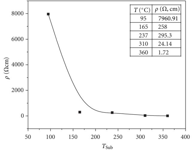
FIGURE 6: Variation of electrical resistivity of  $\text{Bi}_2\text{Se}_3$  as a function of temperature.
