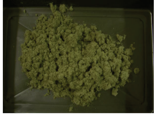
FIGURE 4: Image of the prepared glass fibers.
