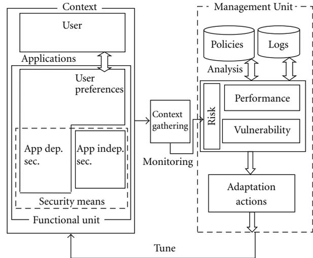
FIGURE 1: SARM components high-level view.
