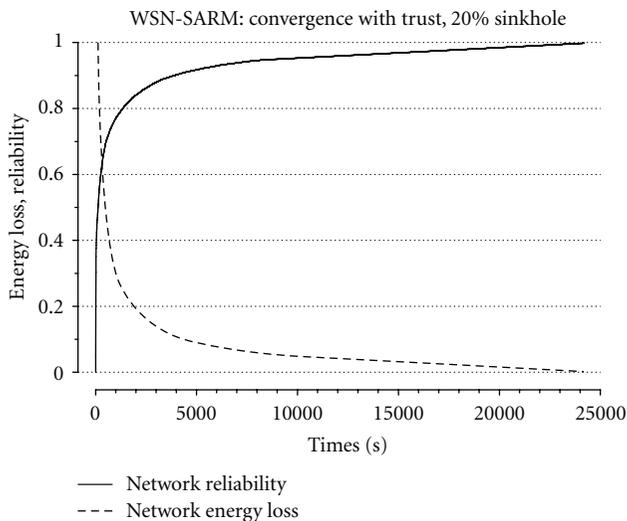
FIGURE 11: Reliability and energy loss of WSN-SARM for the 2nd scenario.
