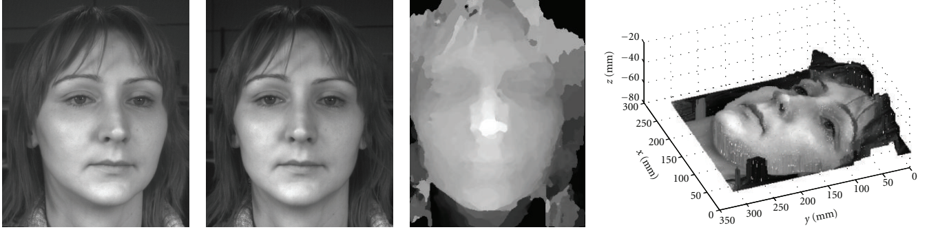
FIGURE 8: Disparity results for the stereo pair Sanja , taken at the vision laboratory of Signals and Systems Group, University of Twente. Size of each image is 781 \times 641 pixels. Disparity range is 0 to 40. (a) Left stereo image, (b) right stereo image, (c) disparity map corresponding to the right image, and (d) depth map with texture overlay.
