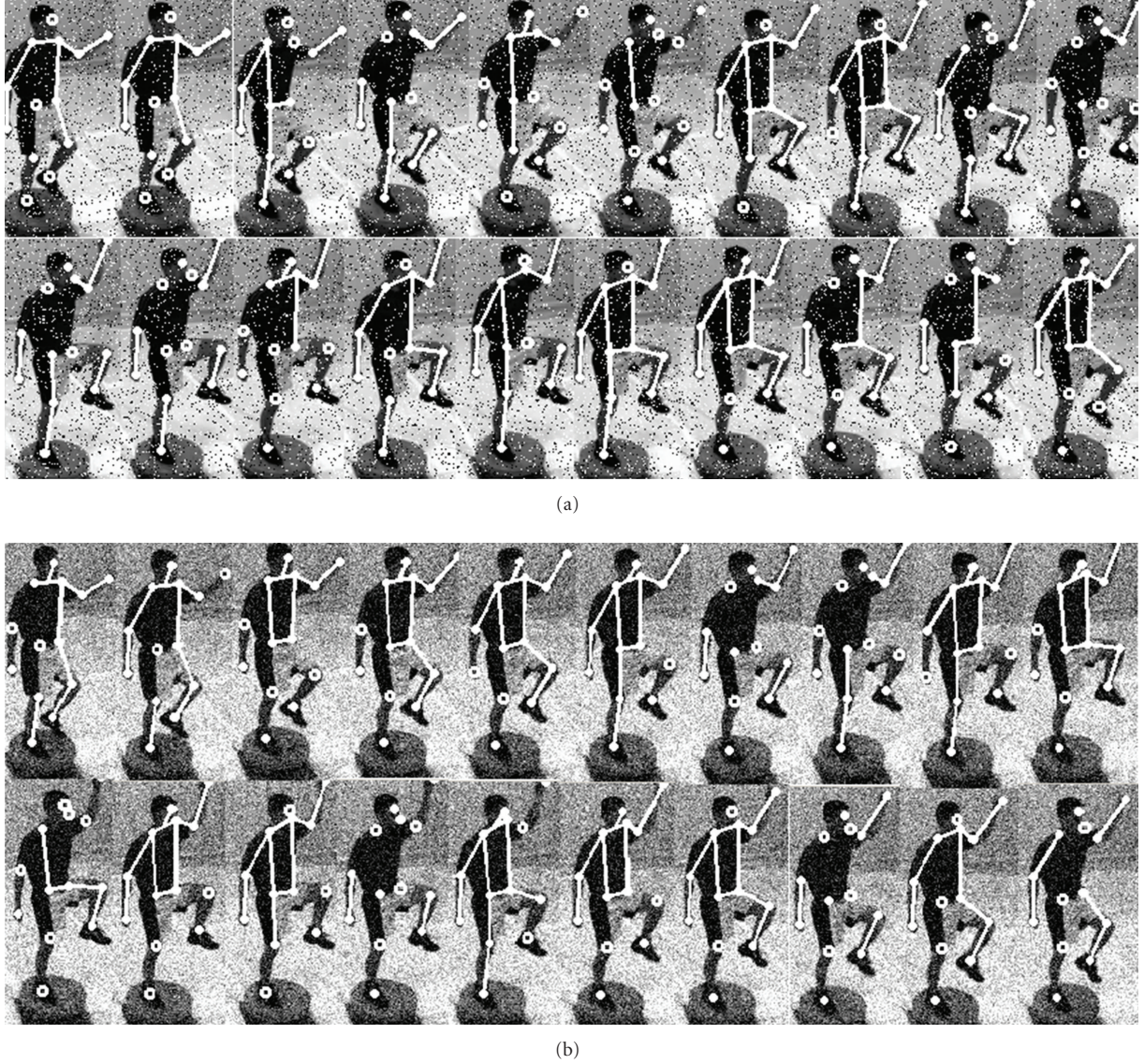
FIGURE 9: Tracking results of the proposed algorithm in the noisy environments. (a) Noisy image with 10 percent salt and pepper noise, (b) images with Gaussian noise of SNR = 10 dB.
