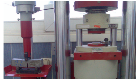
FIGURE 5: Materials testing system, MTS-810 machine.
