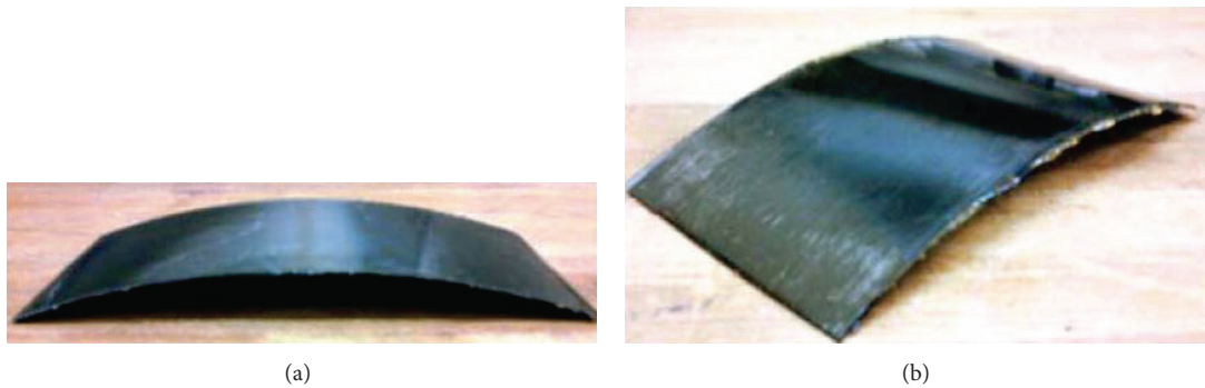
FIGURE 9: Rectangular and square cured room temperature [0_2/90_2] laminates.
