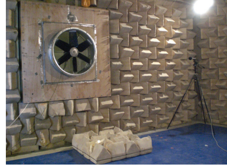
FIGURE 2: Test rig set-up in the semianechoic room.
