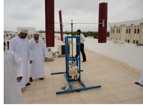
FIGURE 3: Vertical axis wind turbine setup at SCT.
