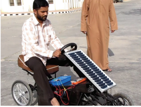
FIGURE 1: Solar-powered electric car experimental setup.
