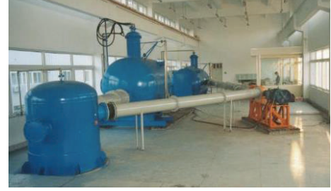
FIGURE 10: Test system of model pumping system.
