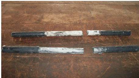
FIGURE 5: Failure pattern of the composite bar under tensile loading.
