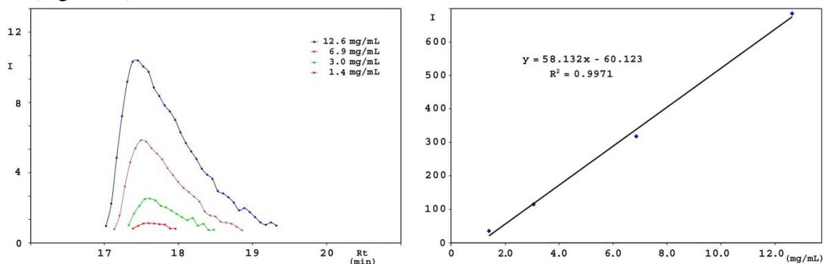
Figure S1. Calibration of the SEC-NMR method. "I" on the Y-axis stays for integral in the individual  $^1\text{H}$  NMR spectra (left) and overall integral obtained by numerical integration (right).
