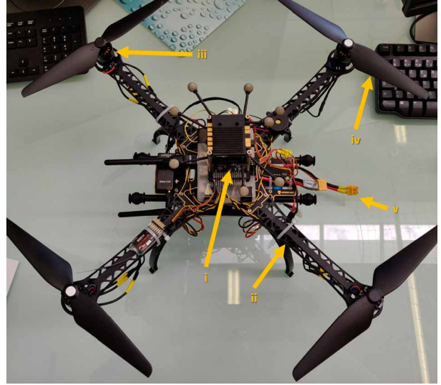
FIGURE 1: Multirotor in quad X configuration with visible components of the propulsion chain. (i) Flight Controller, (ii) ESC (under arm), (iii) BLDC Motor, (iv) propeller, and (v) battery connector.
