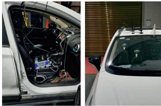
FIGURE 4: Layout of vehicle-mounted units and antenna placement.
