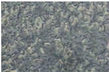
FIGURE 2: Polarising optical microscope textures of SmC schlieren at 139.6°C exhibited by the compound C-11.
