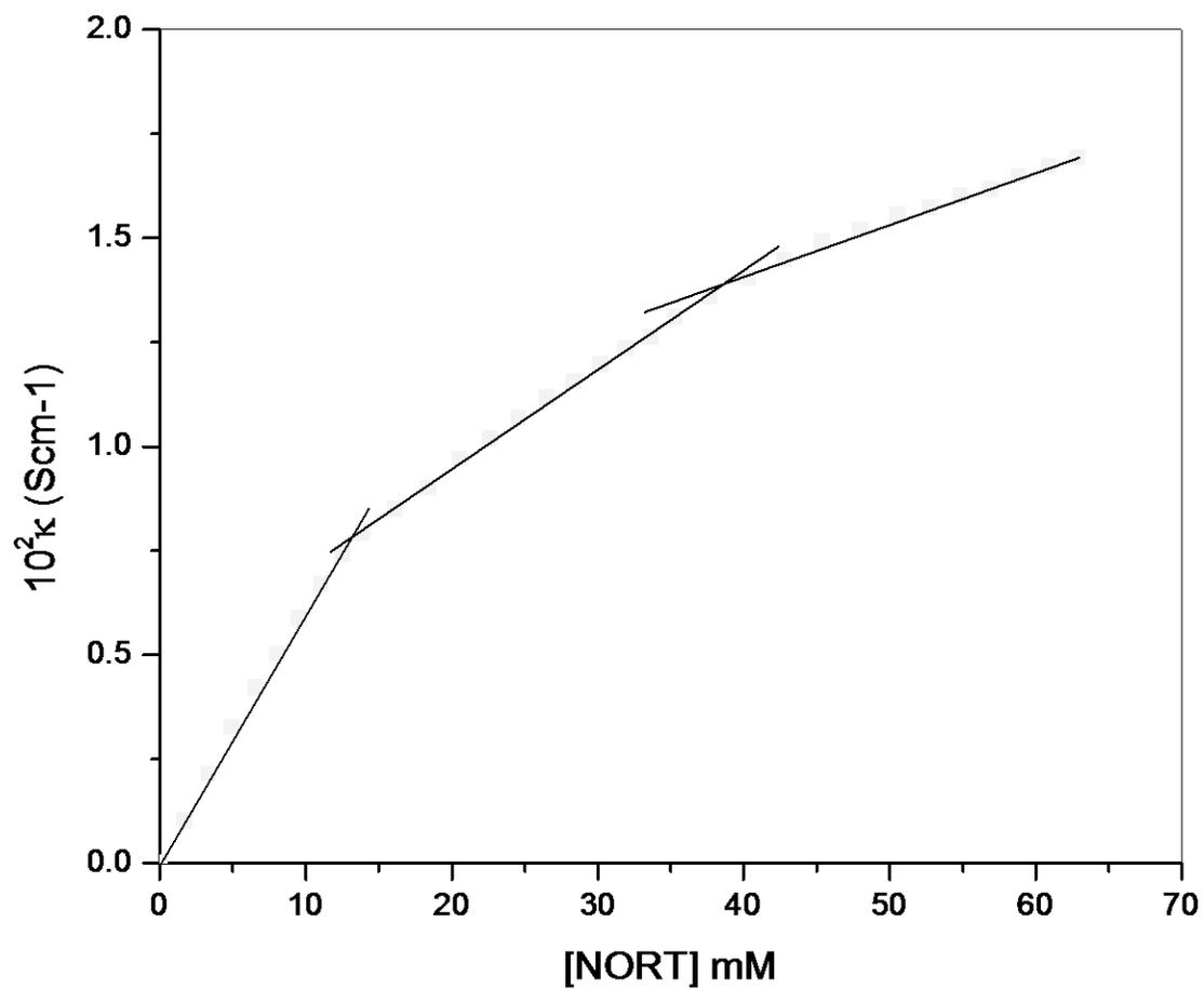
**Fig. S1.** Plot of specific conductivity ( $\kappa$ ) versus [NORT] at 25 °C.
