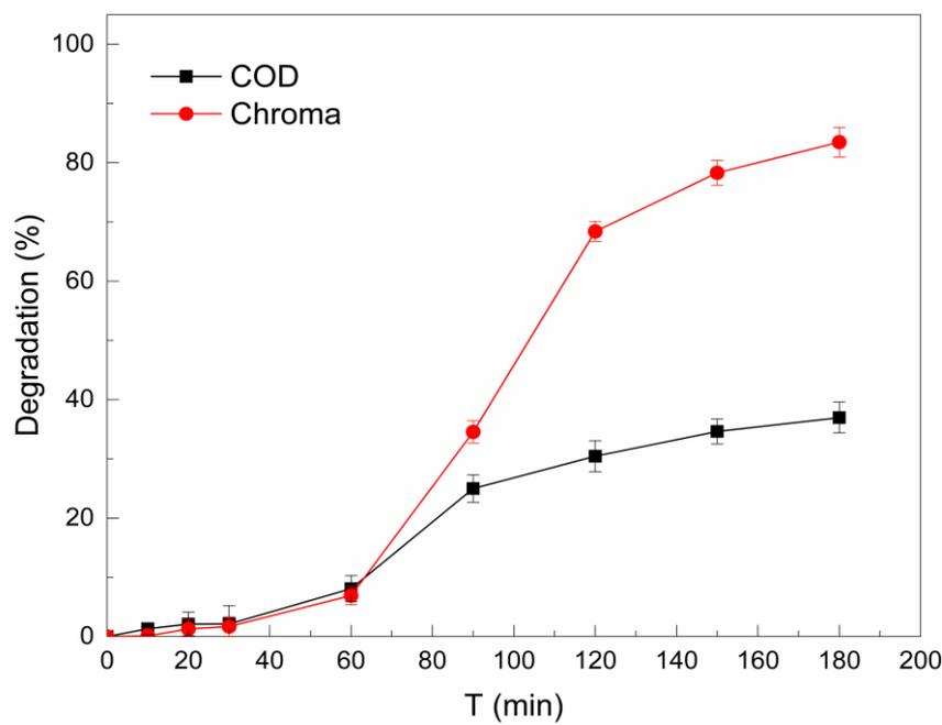
FIGURE.1S: Relationship between ozonation effect and reaction time.
