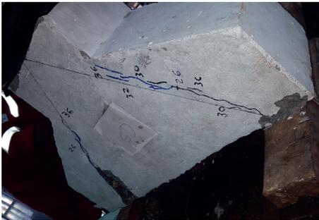
FIGURE 4: The failure mode for corbel specimens.
