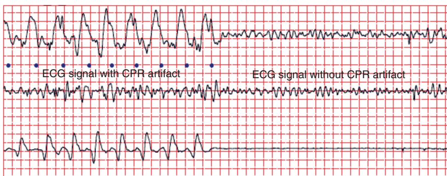
Figure 4. An example of filtering for ventricular fibrillation. The upper trace is the measured ECG signal with/without CPR artifact. The middle trace is the filtered signal. The lower trace is CPR acceleration signal (Reprinted with permission from Tan et al. [33]).
