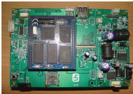
FIGURE 4: Photograph of the base board with core module.
