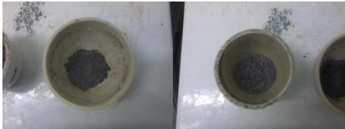
Photograph showing the color/aspect of the pyrolytic products PS-b-4-PVP•(VCl<sub>3</sub>)<sub>y</sub> and Chitosan •(VCl<sub>3</sub>)<sub>y</sub> in ratio 1:5
