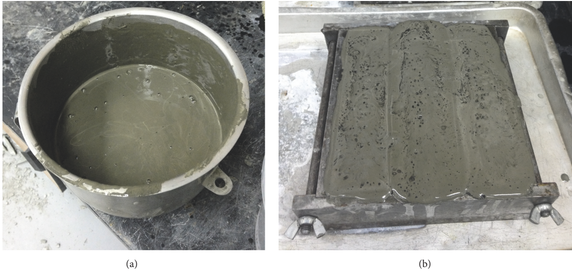
FIGURE 1: (a) Mixing of cement composite batch. (b) Sample of casted specimens including CNTs.
