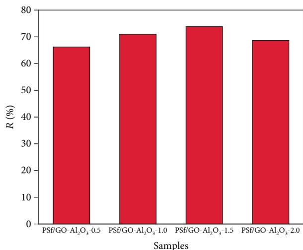
FIGURE 9: Rejection of PSf/GO-Al<sub>2</sub>O<sub>3</sub>-0.5, PSf/GO-Al<sub>2</sub>O<sub>3</sub>-1.0, PSf/GO-Al<sub>2</sub>O<sub>3</sub>-1.5, and PSf/GO-Al<sub>2</sub>O<sub>3</sub>-2.0 membranes (test conditions: operating pressure of 0.87 bar at ambient temperature, feed emulsion: 450 mg/L, and pH = 7).
