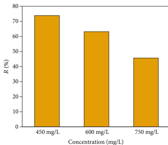
FIGURE 11: Rejection of PSf/GO-Al<sub>2</sub>O<sub>3</sub>-1.5 membrane with different emulsion concentrations (test conditions: operating pressure of 0.87 bar at ambient temperature and pH = 7).
