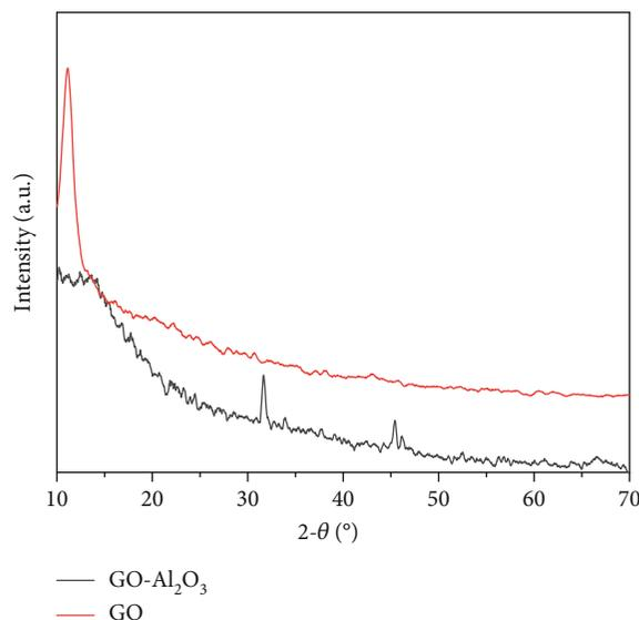
FIGURE 1: XRD patterns of GO and GO- $\text{Al}_2\text{O}_3$  samples.
