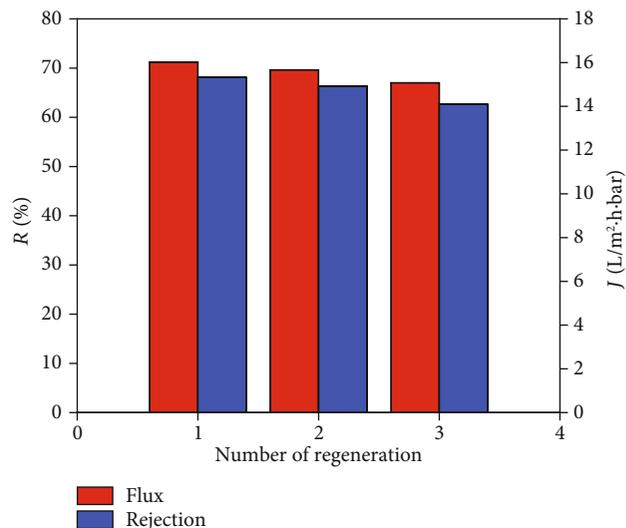
FIGURE 14: Rejection and permeate flux of PSf/GO- $\text{Al}_2\text{O}_3$ -1.5 membrane after three cycles in 30 min (test conditions: operating pressure of 0.87 bar at ambient temperature and feed emulsion: 450 mg/L).
