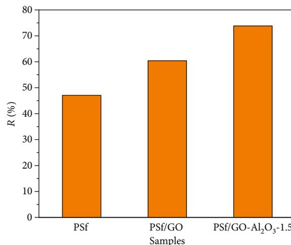
FIGURE 7: Rejection of the PSf, PSf/GO, and PSf/GO- $\text{Al}_2\text{O}_3$ -1.5 membranes (test conditions: operating pressure of 0.87 bar at ambient temperature and feed emulsion: 450 mg/L).
