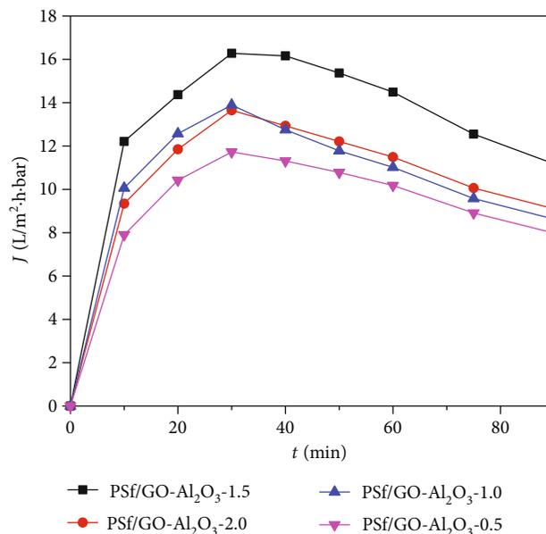
FIGURE 10: Permeate flux of PSf/GO-Al<sub>2</sub>O<sub>3</sub>-0.5, PSf/GO-Al<sub>2</sub>O<sub>3</sub>-1.0, PSf/GO-Al<sub>2</sub>O<sub>3</sub>-1.5, and PSf/GO-Al<sub>2</sub>O<sub>3</sub>-2.0 membranes (test conditions: operating pressure of 0.87 bar at ambient temperature, feed emulsion: 450 mg/L, and pH = 7).
