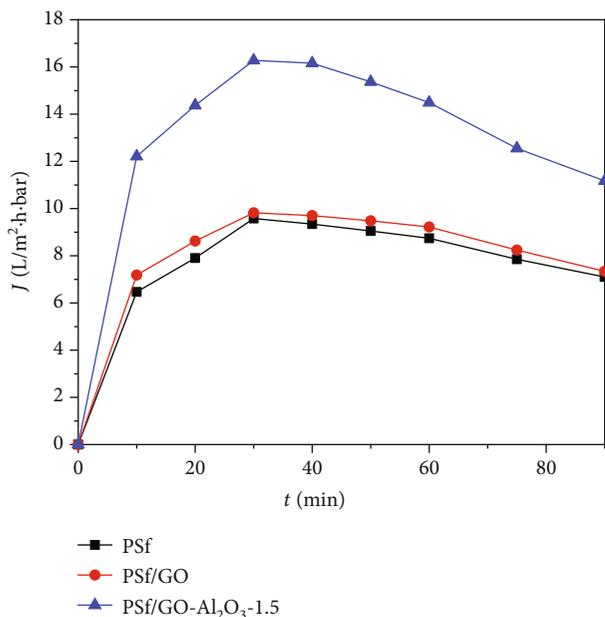
FIGURE 8: Permeate flux of the PSf, PSf/GO, and PSf/GO-Al<sub>2</sub>O<sub>3</sub>-1.5 membranes over time (test conditions: operating pressure of 0.87 bar at ambient temperature and feed emulsion: 450 mg/L).
