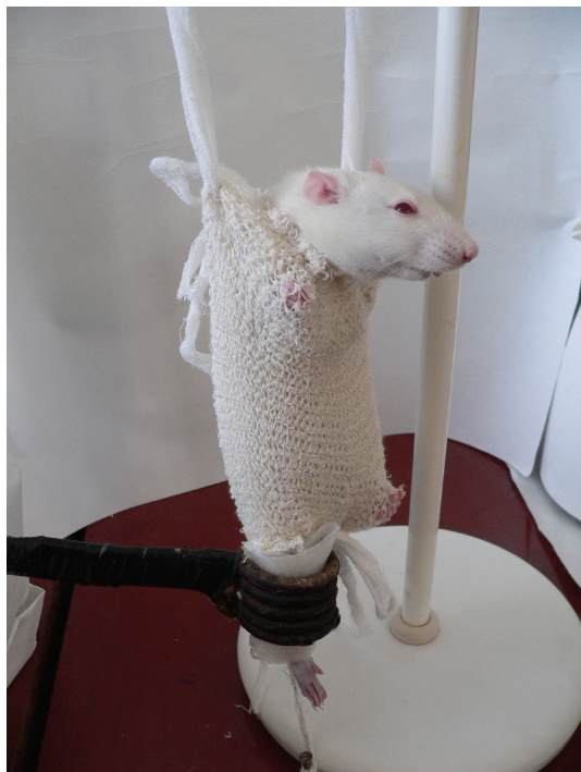
FIGURE 2: Rat is in the net-hammock and the femur is located in the coil of magnetic field generator.
