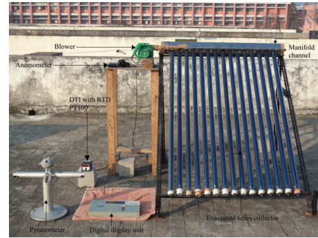
FIGURE 1: Experimental setup of evacuated tube solar air collector.
