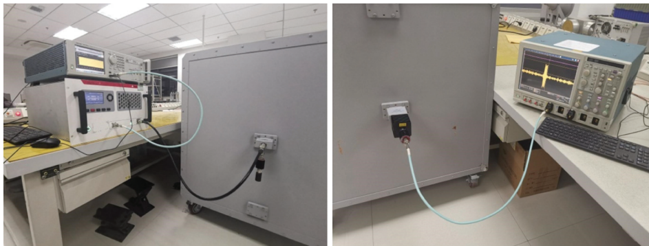
FIGURE 7: The fabricated cavity and the HPM pulse obtained system according to the principle of Figure 6.
