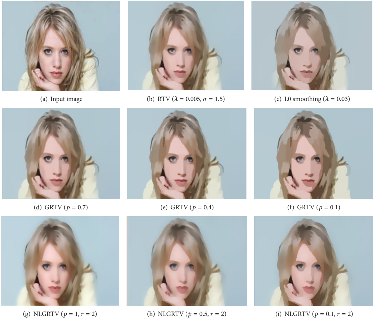
FIGURE 6: Effect of varying parameters. Smaller p -values give more prominent edges sharpening results and nonlocal way in favor of preserving shade information.
